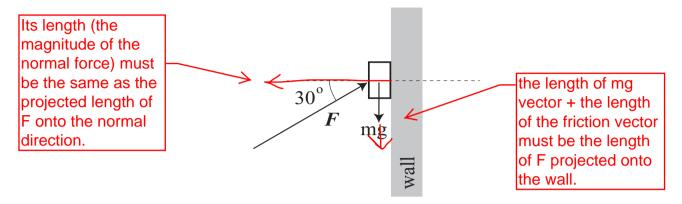
(a) In the above figure already the force F and the gravitational force acting on mass m are drawn. Draw the remaining (two) forces acting on the block to complete the free body diagram in the figure above. (Try to be quantitative, using appropriate lengths of arrows. The vectors already drawn are quantitative.) [5]
