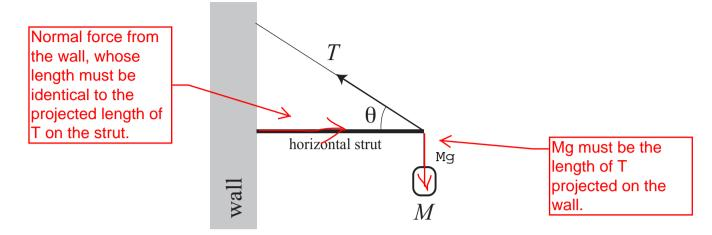
(a) You may assume that the force from the wall on the strut is horizontal. Draw in the figure all the forces (actually, two more forces) acting on the strut. The tension in the string is already drawn.[5]
