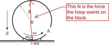
(a) Suppose R = 1.2 m. What is the force (its direction and magnitude) that the block exerts on the hoop when the block is just passing the bottom? [5]
