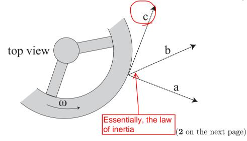
2. An ancient phonogram used a vinyl disk that rotates at a constant rotational speed of 100/3 rpm.
