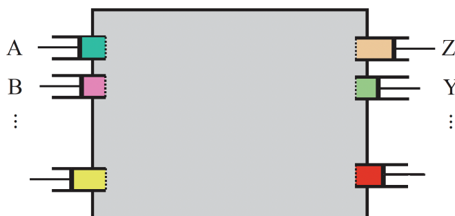
Figure 25.2: Van't Hoff の平衡箱
